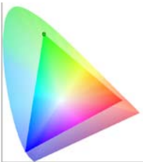
Figure 3. Here Adobe RGB (1998) is plotted. Notice that the red, green, and blue primaries are farther apart than those seen in Figure 2. Since they move farther out from the center, closer to the maximum saturation of human vision, it is fair to say the color gamut is larger than sRGB.
