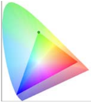
Figure 2. In a similar color plot, the sRGB color space is grafted over the CIE x,y Chromaticity Diagram. The red, green, and blue primaries form the simple triangular shape. The green dot represents the most saturated green (R0/G255/B0).
